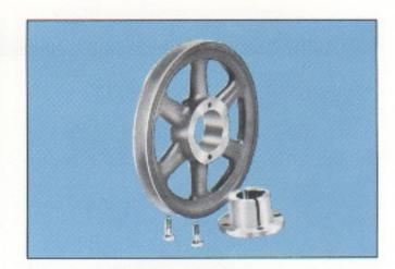
When mounting the Split Taper bushing there is only one position that will work because the keyway on the taper of the bushing must match the keyway on the bore of the companion product. Since Sure-Grip bushings do not have keyways on their tapers, they can be mounted in any of the three or four positions to align the bolt holes.
